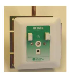
of an inch (1.3 cm to 3 cm). The name of the gas service shall be permanently marked on the outlet bracket and the outlet. The outlet's rough-in supply tube shall be a 7 inch (18 cm) length of 1/2 O.D. copper Type K for all gas services and labeled with the name of the gas service.
